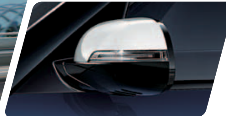
Outside mirror electrically folding (SX only), adjustable and heated side mirrors are available in body colour or high-gloss black finishes depending on trim level.
