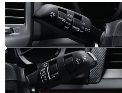
Headlamp control and automatic washer switches
